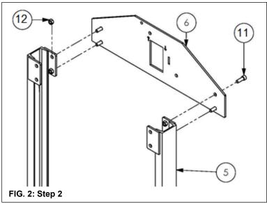
Step 2: As shown in FIG. 2, fasten a jack plate (6) onto vertical supports (5) using bolts (11) and Nylock nuts (12). Labels on the jack plate must face outward to be visible to users.
