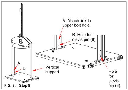
Step 10: Lock the roll-out tray to the frame. Insert clevis pins (6) through the bottom holes (B) of the vertical supports and through the hole on the roll-out tray when moving unit. See *F/G*. 8.
