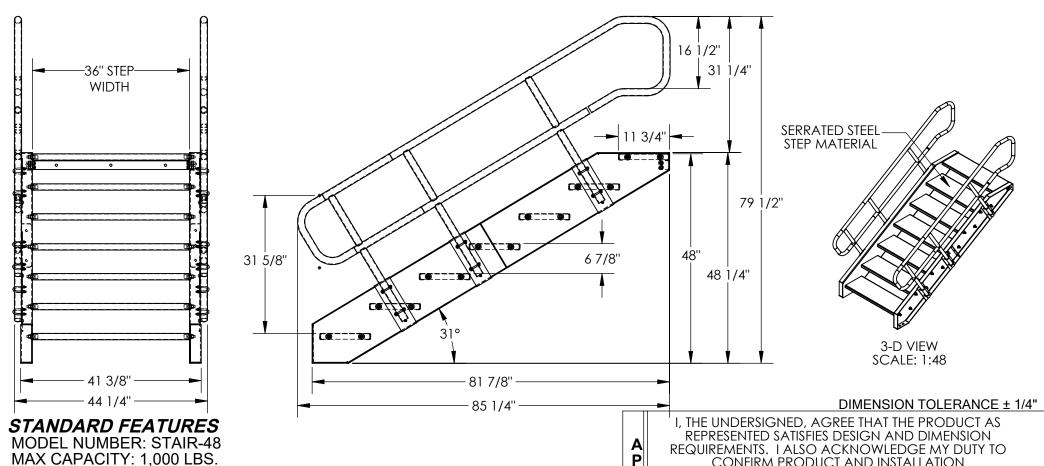
MAX CAPACITY: 1,000 LBS. STANDARD STEP WIDTH: 36" STEP HEIGHT SPACING: 6 7/8"
