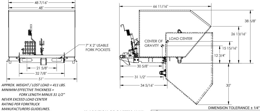
DO NOT USE THIS FORK TRUCK ATTACHMENT IF LOAD WILL EXCEED FORK TRUCK MANUFACTURER'S LOAD CENTER RATING
