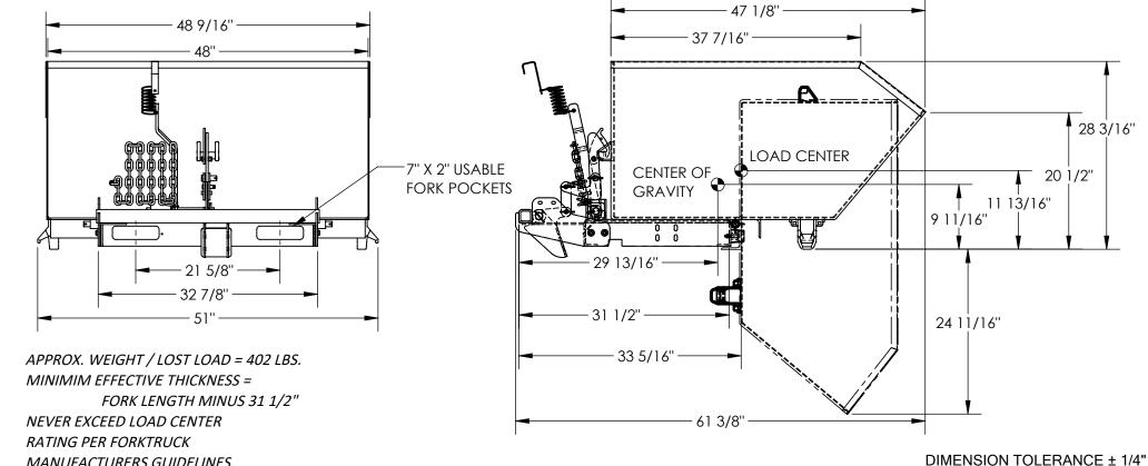
MANUFACTURERS GUIDELINES. DO NOT USE THIS FORK TRUCK ATTACHMENT IF LOAD WILL EXCEED FORK TRUCK MANUFACTURER'S LOAD CENTER RATING
