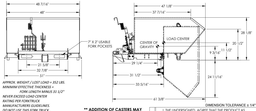
CHANGE WEIGHT CAPACITY ATTACHMENT IF LOAD WILL **BASED ON CASTER RATING** EXCEED FORK TRUCK MANUFACTURER'S LOAD CENTER RATING
