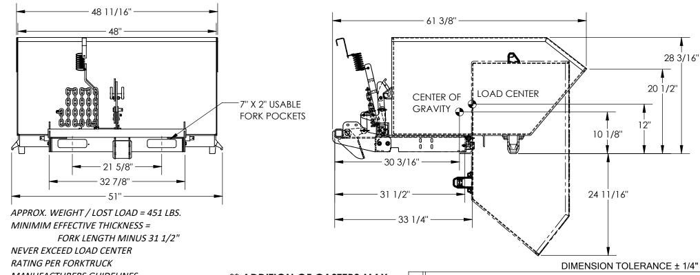
MANUFACTURERS GUIDELINES. DO NOT USE THIS FORK TRUCK ATTACHMENT IF LOAD WILL EXCEED FORK TRUCK MANUFACTURER'S LOAD CENTER RATING
