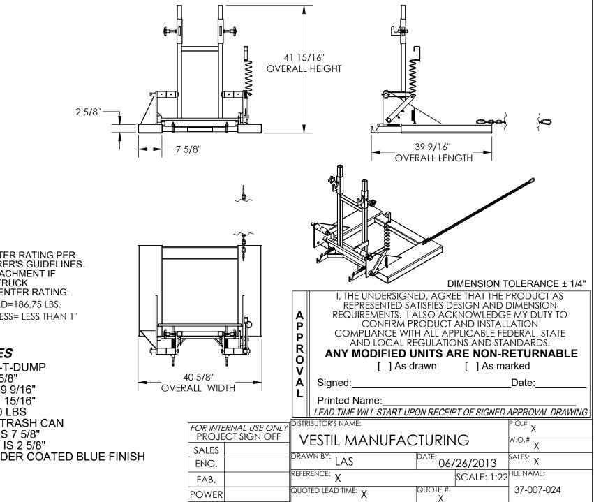
NEVER EXCEED LOAD CENTER RATING PER FORK TRUCK MANUFACTURER'S GUIDELINES. DO NOT USE HIS FORK ATTACHMENT IF LOAD WILL EXCEED FORK TRUCK MANUFACTURER'S LOAD CENTER RATING. APPROX. WEIGHT/ LOST LOAD=186.75 LBS. MINIMUM EFFECTIVE THICKNESS= LESS THAN 1"
