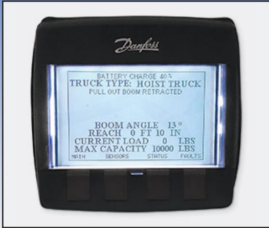
Rated Load Limiter Automatically detects attachment and adjusts loading parameters
