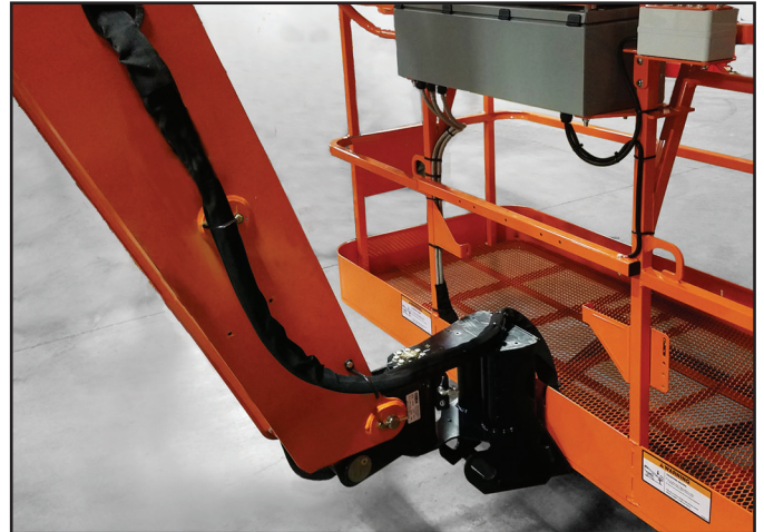
Bailey's Platform Control Box
